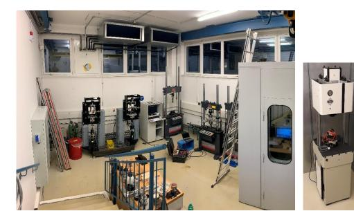
3 MTS axial test benches 3 MTS bending test benches RUMUL 150 kN from 45-260 Hz Elevated temperatures up to 1000 deg. C Climatized room Argon fire extinguisher
