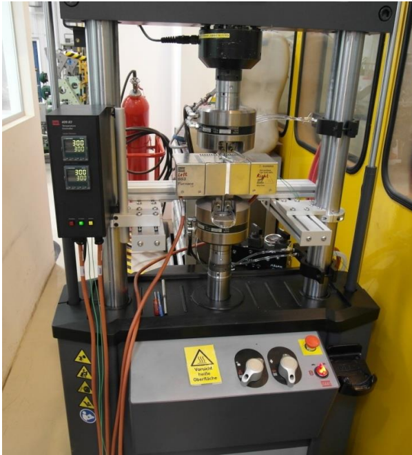
Tension/compression test rig with heat chamber
